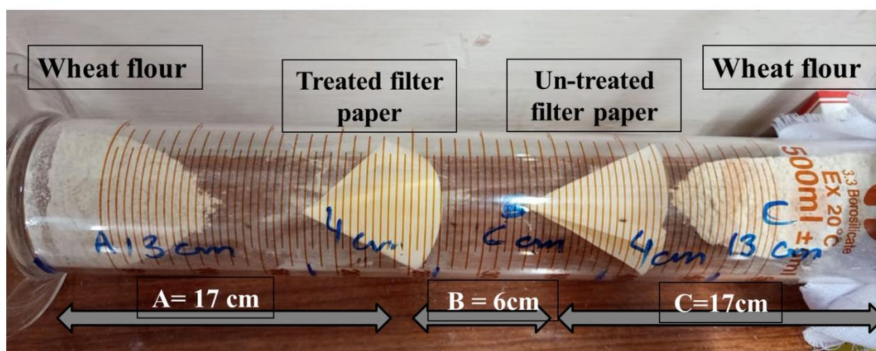
**Fig. 1.** Systematic diagram of cylinder trap for evaluating repellent efficacy of medicinal oils against *Tribolium castaneum*.
